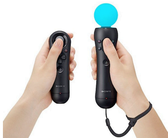
Figure 1.25 – The PlayStation Move controller (right) and the Navigation controller. The glowing orb on top of Move is captured by the Eye camera as an active marker to detect its position in space 144 .
