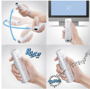
Figure 1.23 – The Wii Remote detects motion using a three-axis accelerometer 139 .
