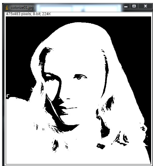
Figure 3.10. Good silhouette after thresholding.
