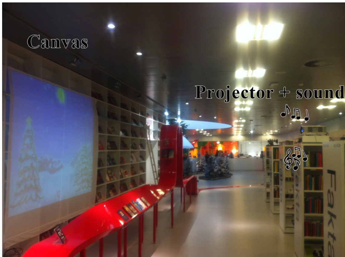
Figure 6.18. Since the speakers are inside the projector, audio will draw attention to the wrong side.
