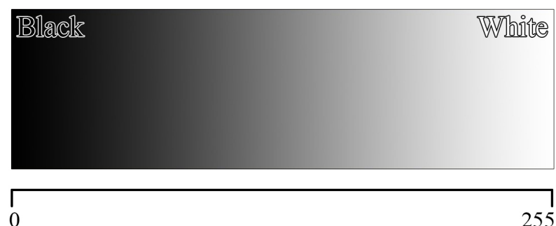
Figure 3.5. Image illustrating the 256 different gray-level values of an 8 bit picture.
