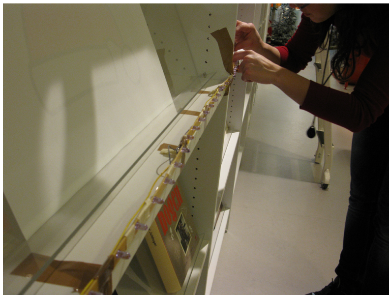
Figure 6.3. The LEDs are put on a long strip at 4 centimetres intervals.
