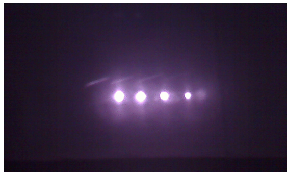
Figure 4.4. The LEDs have been sanded down in progressive order from left to right.
