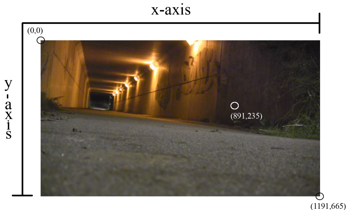
Figure 3.6. The pixel values are stored in a coordinate system. Note that the Y-axis is reversed.
